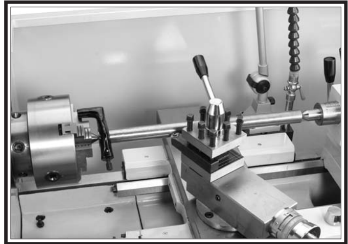
Figure 46. Example photo of stock mounted between the centers.
